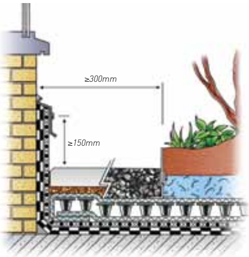
Detail 3. Facade with an opening
